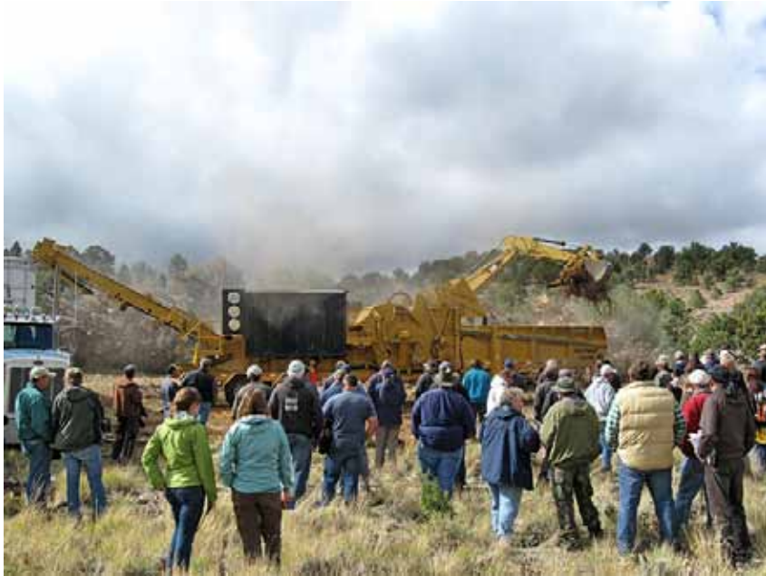
The CBI Magnum Force 6400 demonstrates how quickly it can fill a trailer with chips as participants observe the equipment in action.
