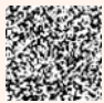
Fig. 2. A sample of the watermark pattern. The pattern follows the distribution N(0,1) . For an M \times M pixel image, the size of the watermark is (M/8) \times (M/8) pixels.
