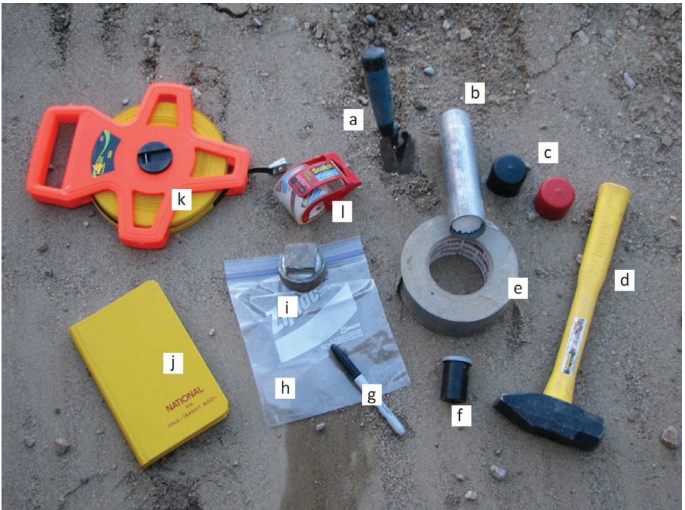
FIGURE 3. Typical sample-collection gear used for luminescence dating. Items identified include: (a) trowel (or field knife or small shovel) for clearing back of sediments from the face of the trench or outcrop and collection of sediment for dose-rate samples; (b) OSL sampling tube (metal or other opaque material) sharpened at one end and pre-loaded with a styrofoam plug on the sharpened end to limit sediment shaking during pounding; (c) end caps for sample tube (tin foil and duct tape can be substituted if not available); (d) sledge hammer for pounding in sample tube (rubber mallets and light field hammers are not recommended for most sediment types); (e) duct tape to seal ends of tubes; (f) film canister for water-content samples (triple-bagged zip-bags or other airtight containers also acceptable); (g) permanent marker for labeling samples; (h) one-quart (ca. 1 liter) zip-seal bag half-filled for dose-rate sample collection; (i) pounding cap (a 2-in outside threaded plug is shown; it is important not to use pounding caps that fit tightly on tubes or that have internal threads as they can get permanently seized onto pipes); (j) field note book to document stratigraphic context and GPS location and elevation; (k) measuring tape to determine sample depth; and (l) clear packing tape to cover labels so they do not get worn off during shipping. Additional material in a sampling toolkit could include tin foil for wrapping samples and securing tube ends if end caps are not available, a camera to document sample placement, and light-proof tarps for use if modified sample collection is necessary (e.g., for coarse-grained deposit or sampling under rocks).
