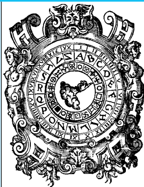
This Renaissance crypt-analysis instrument works by rotating the inner disk against the stationary outer disk.
