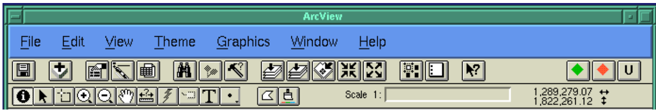
Figure 2: The View Document GUI for the Chunky Monkey Version of the Link. The Button Bar contains three additional buttons: 1) a green diamond that initiates the link; 2) a red diamond that terminates the link; and 3) a “U” icon that updates the CDF plots after region definitions have been changed. The Tool Bar contains two additional tools: 1) a region definition tool that allows regions to be defined for which CDFs will be calculated; and 2) a brush tool that allows transient brushing in ArcView.
