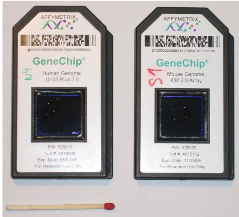
Figure 1: Affymetrix microarrays: U133 Plus 2.0 (left), array for the Human Genome; 430 2.0 Array (right), array for the Mouse Genome. Image taken from http://en.wikipedia.org/wiki/File:Affymetrix-microarray.jpg , April 16, 2009.
