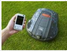
Husqvarna's autonomous Automower 260 ACX calls for help via SMS
